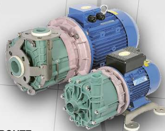
ROUTE range Installed powers: kW 0,55÷7,5 Bodies materials: GFR/PP - CFF/E-CTFE • Magnetic drive • Sealed
