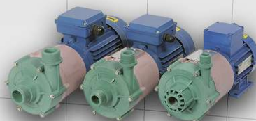
AM range Installed powers: kW 0,18÷0,55 Bodies materials: GFR/PP - E-CTFE • Magnetic drive
